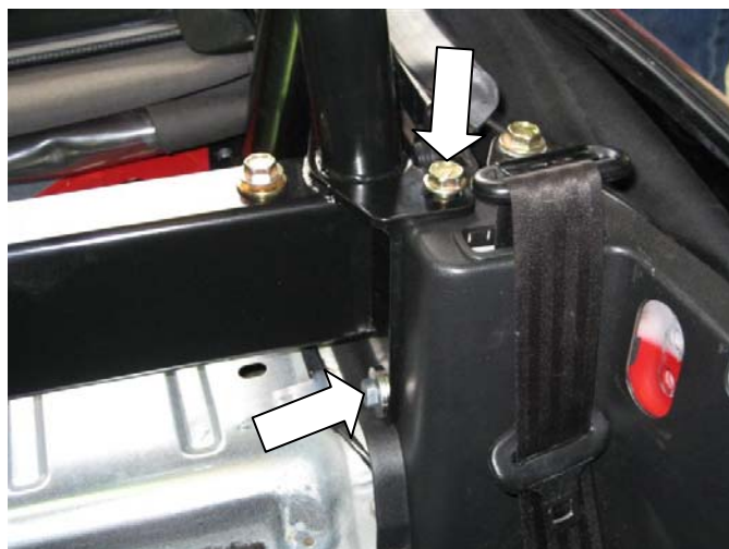
Two bolts installed on the left side of the rollbar
