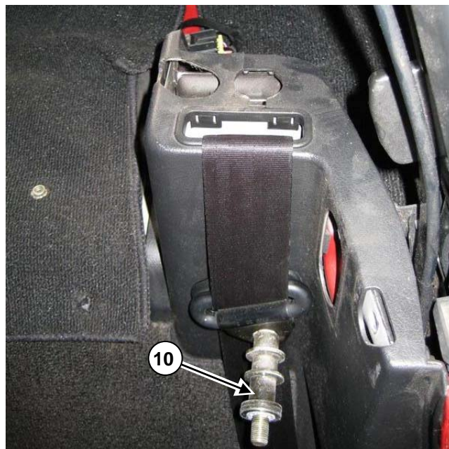
Left side upper seatbelt mounting bolt (10) removed
