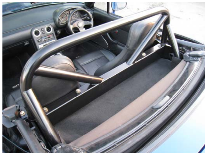
MX-5 Plus rollbar installed
