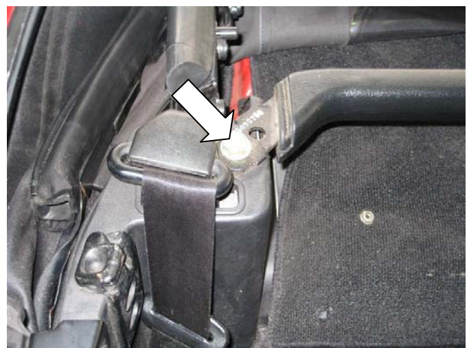
Right side mounting bolt for the cross brace
