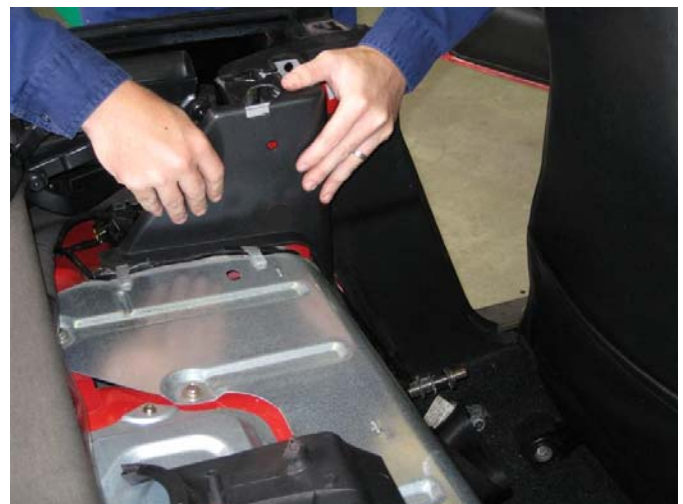
Left side plastic trim being removed from the vehicle
