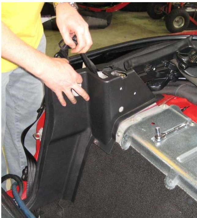
Insert the seatbelt through the plastic trim on final installation
