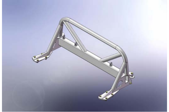
Single Hoop Style Rollbar with mounts and harness points installed
