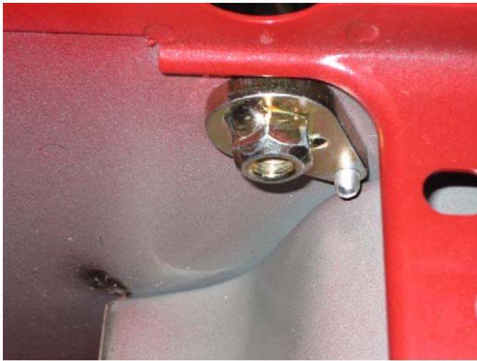
View inside the seatbelt cavity showing the mounting plate riveted to the body
