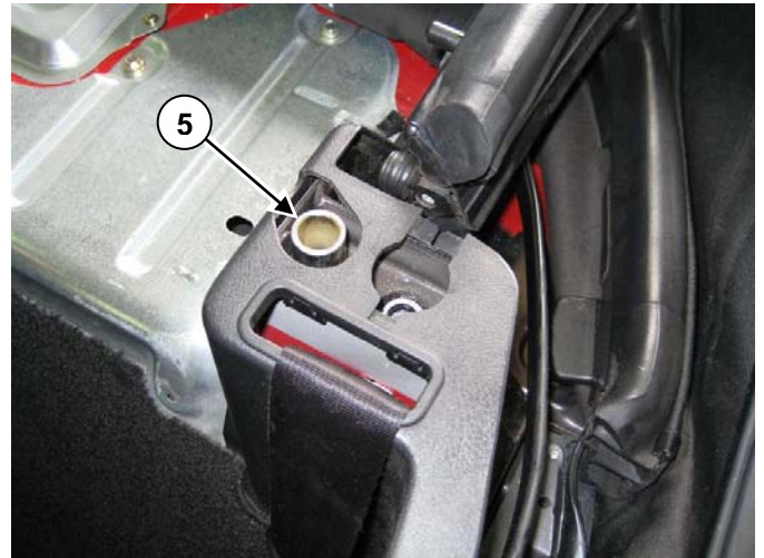
Spacer installed in the vehicle (plastic trim shown)
