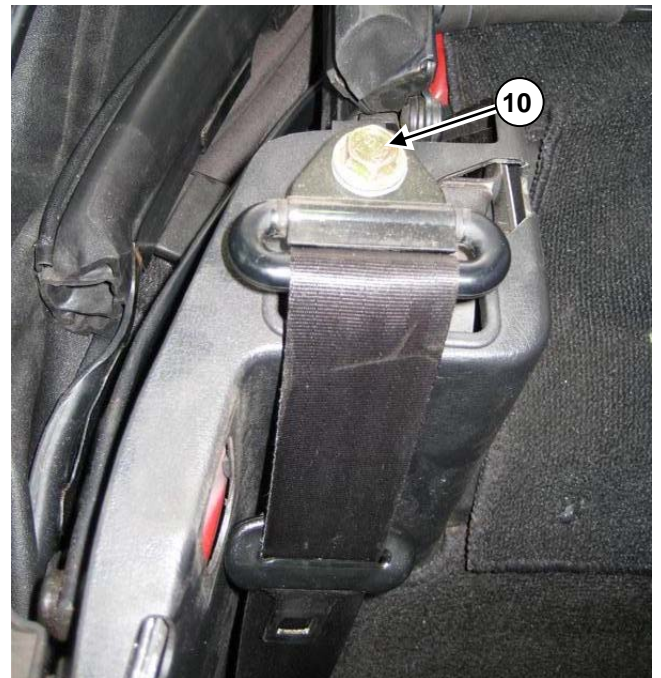
Reinstall the upper seatbelt mounting bolt (10)
