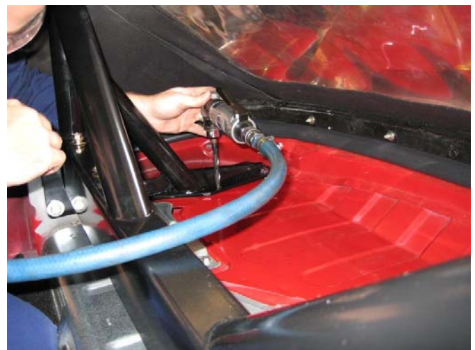
Drill holes in the rear parcel shelf using the rollbar holes as a template
