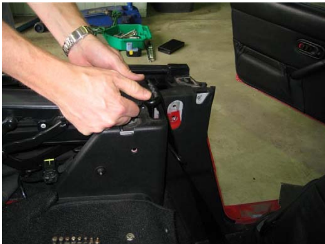
Pull off the plastic cover to expose the upper seatbelt mounting bolt
