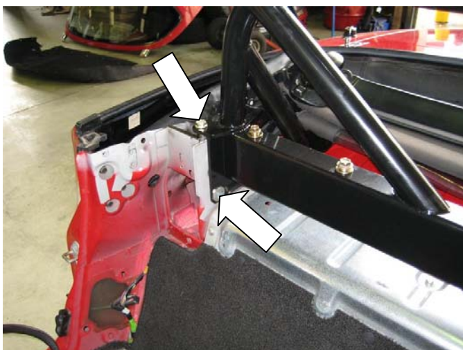
Rollbar mounting hardware installed in two places on the right side of the vehicle (plastic trim not shown)
