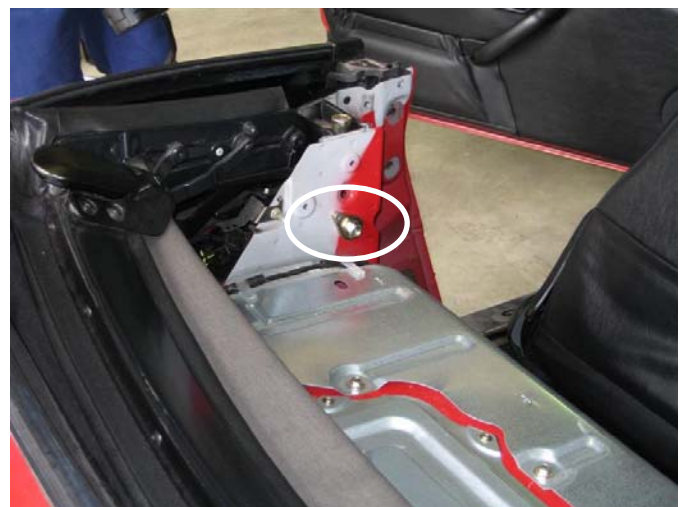
Mounting plate bolted to the body of the vehicle
