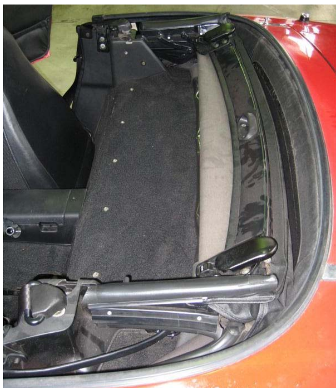
Cross brace removed from vehicle
