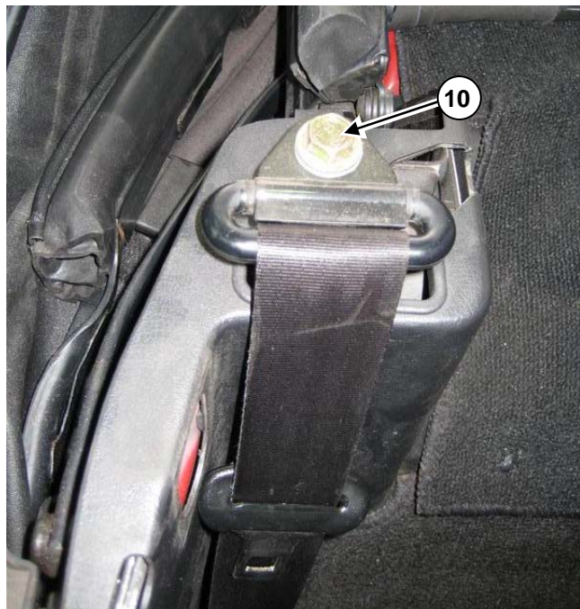
Upper seatbelt mounting bolt (10)
