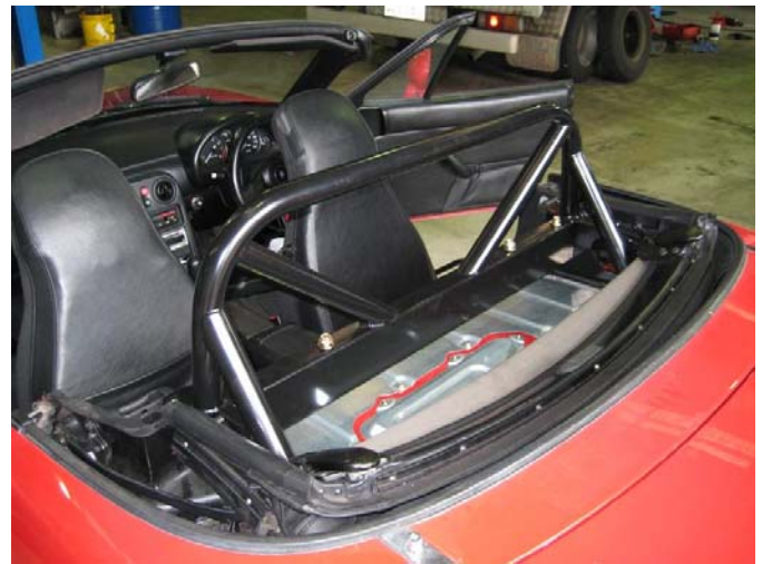
Rollbar positioned in the vehicle
