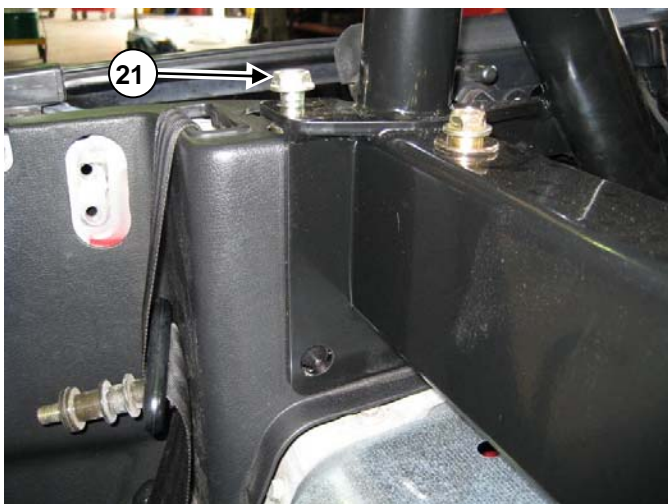
Remove bolt (21) from each end of the rollbar
