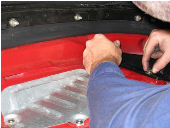
Right side mounting plate (24) orientated for bolting
