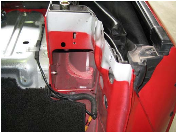
Seatbelt coil removed from housing
