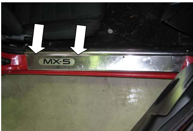
Install and tighten screws from door sill
