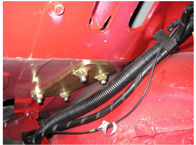
Mounting plate with four bolts installed
