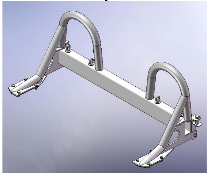
TT Style Rollbar with mounts and harness points installed
