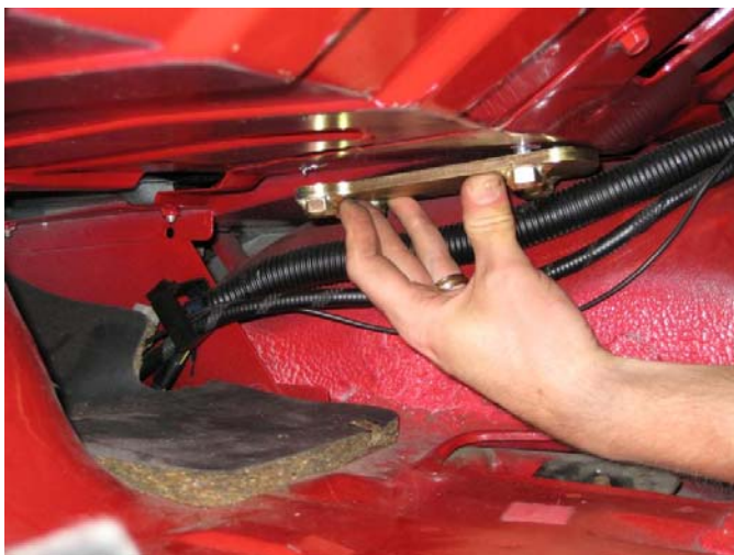
Insert bolts from inside the vehicle whilst the mounting plate is being held in position via the boot
