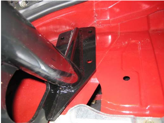
Foot pad aligned with the rear parcel shelf
