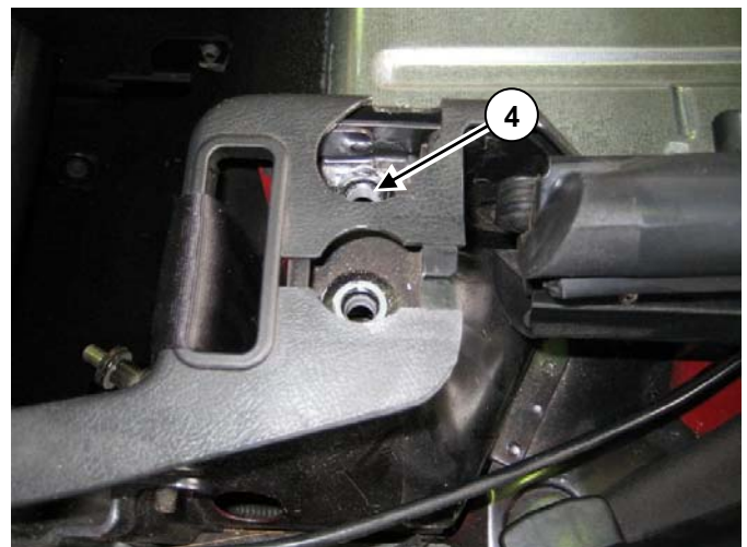
Existing hole in vehicle (4) exposed after removal of the cross brace
