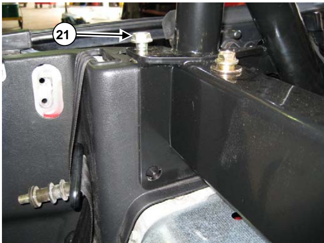
Bolt (21) installed in the right side of the rollbar
