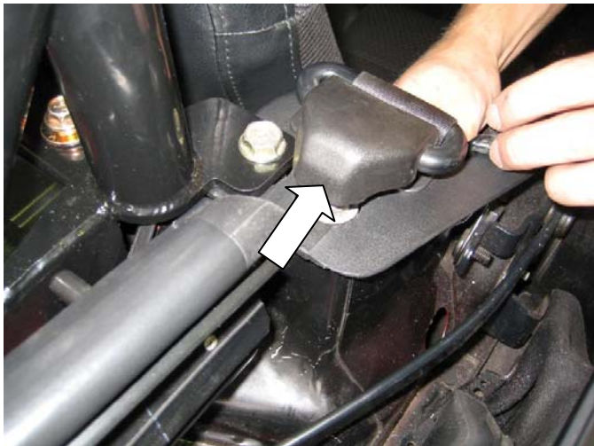
Upper seatbelt mounting bolt (10) installed and the plastic cover fitted
